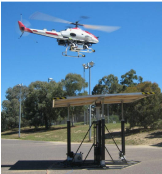
Figure 9: UNSW @ADFA R-Max Hovering over a Moving Deck Simulator.
